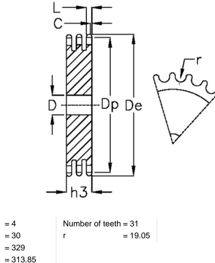
C = 4 D = 30De = 329Dp = 313.85For chain size =  $1 \frac{1}{4} \times \frac{3}{4}$ For chain type = 20 B-3h3 = 91L = 18.2
